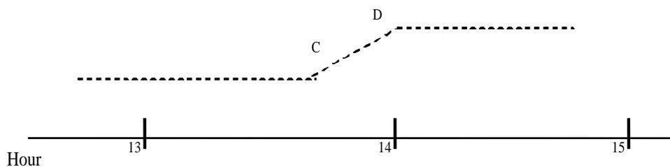
If for any reason the schedule change cannot be achieved in one full hour of ramping (i.e., MW change greater than the applicable energy response rate times 60 minutes), RTD nevertheless ramps the basepoint sufficiently fast to reach the new schedule in one hour and the unit will be responsible for buying replacement energy to make up the difference.
