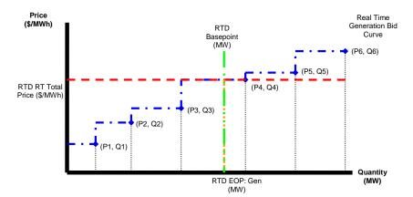
In the diagram below, however, the RTD interval LBMP intersects the given Generation Bid block on a horizontal line; however, the Generator was Base Pointed beyond its economics. In this case, the Generator's EOP is equal to the higher Generation Block MW (i.e.,  $Q_4$ ) of the block where the RTD interval LBMP intersects the Generation Bid.
