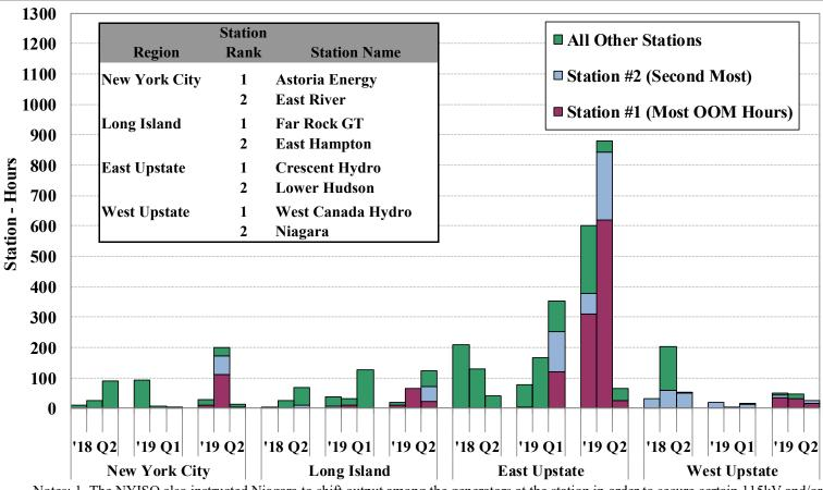
Notes: 1. The NYISO also instructed Niagara to shift output among the generators at the station in order to secure certain 115kV and/or 230kV transmission facilities in 382 hours in 2018-Q2, 517 hours in 2019-Q1, and 806 hours in 2019-Q2. However, these were not classified as Out-of-Merit in hours when the NYISO did not adjust the UOL or LOL of the Resource.
